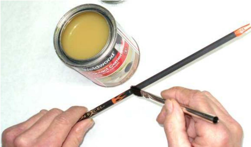
**Step 5) Apply contact cement to the entire fletching area of the shaft.**
