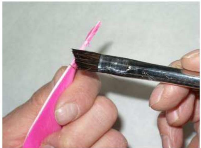
**Step 7) Apply contact cement to the base of each feather.**
