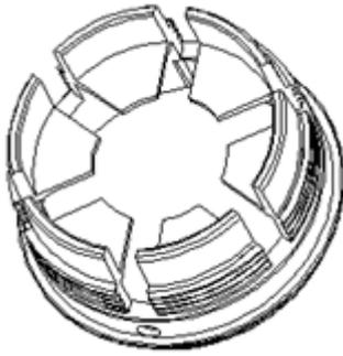
**Built-in chuck** : this unit, fixed on the ocular, is coordinated with the chuck screw ring for contracting and tightening. Its inside circle, matched with different lantern rings, is applicable for various ocular connection.
