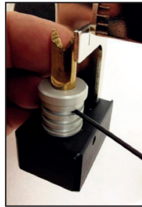
2. Lift the locator barrel till you can reach the set screw.
