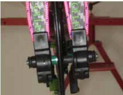
3: Align the ropes and close the lever until the lock engages.
