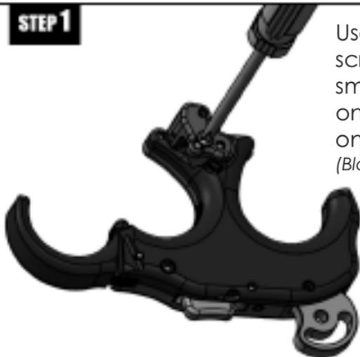
Use a small Phillips head screwdriver to remove the small **silver** panhead screw on the side with only one screw.
